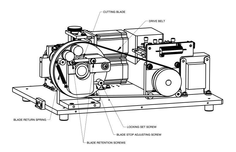
(SHOWN WITH COVER, HOUSING, GUARD, EXIT BUSHING AND EXIT BUSHING SUPPORT REMOVED)
