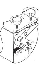
2) Adjust pressure on wire until wire can be stripped without breakage.
