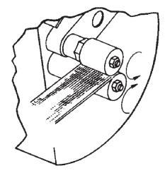
Wheels should be dressed whenever the performance deteriorates. Regular dressing will increase wheel life and production. Wheels may be used to within 1/8" (3.2mm) of their arbor hole.
