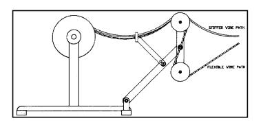
and support arm by loosening the screw to raise or lower the wire path.
