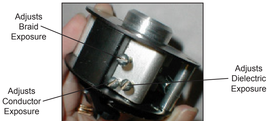
CUTTER HEAD ADJUSTMENT SCREWS
