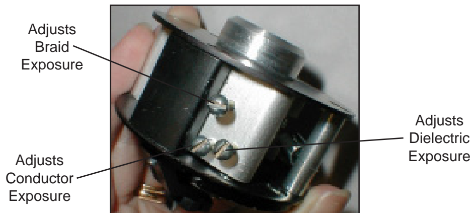
CUTTER HEAD ADJUSTMENT SCREWS
